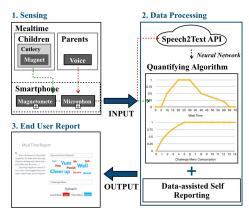
Figure 2. System Block Diagram of MAMAS
